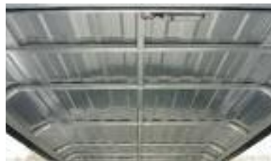
TIG Welded Super Cage Roof Integrated Construction
