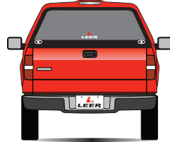
180CC Recessed Dark Tint Rear Door with Double T-Handles (Standard)
